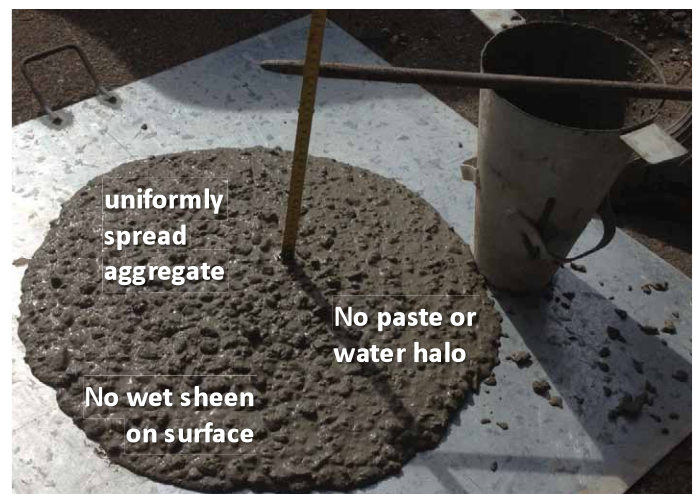
FIGURE A.4: Slumped concrete of Visual Stability Index VSI class 0 (according to ASTM C1611)
